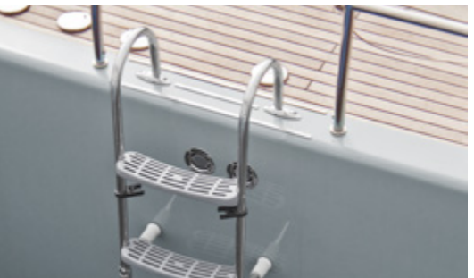
Stainless steel removable ladder at rail gate
