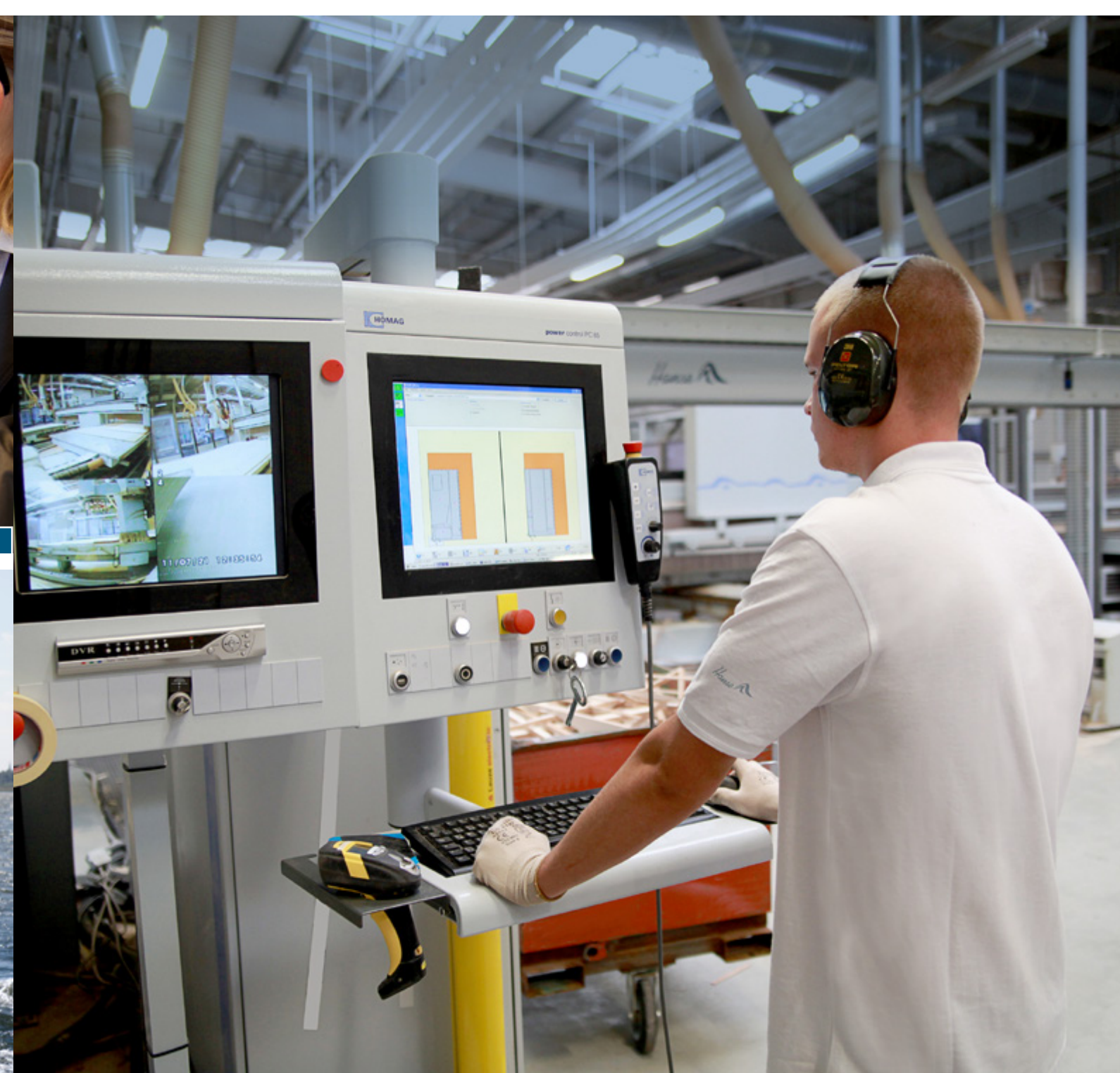
4 Before our carpenters build the interior of a HANSE 385, wood panels are prefabricated using computer control.
