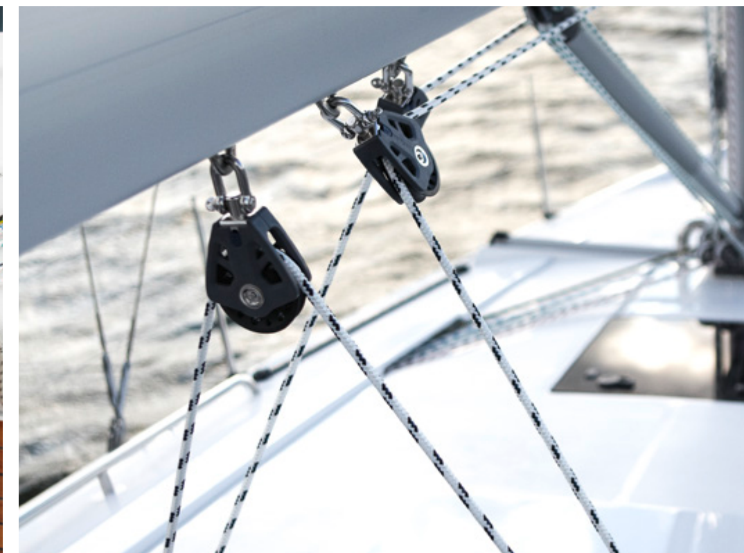
5 German mainsheet system leads aft to helmsman at both sides.
