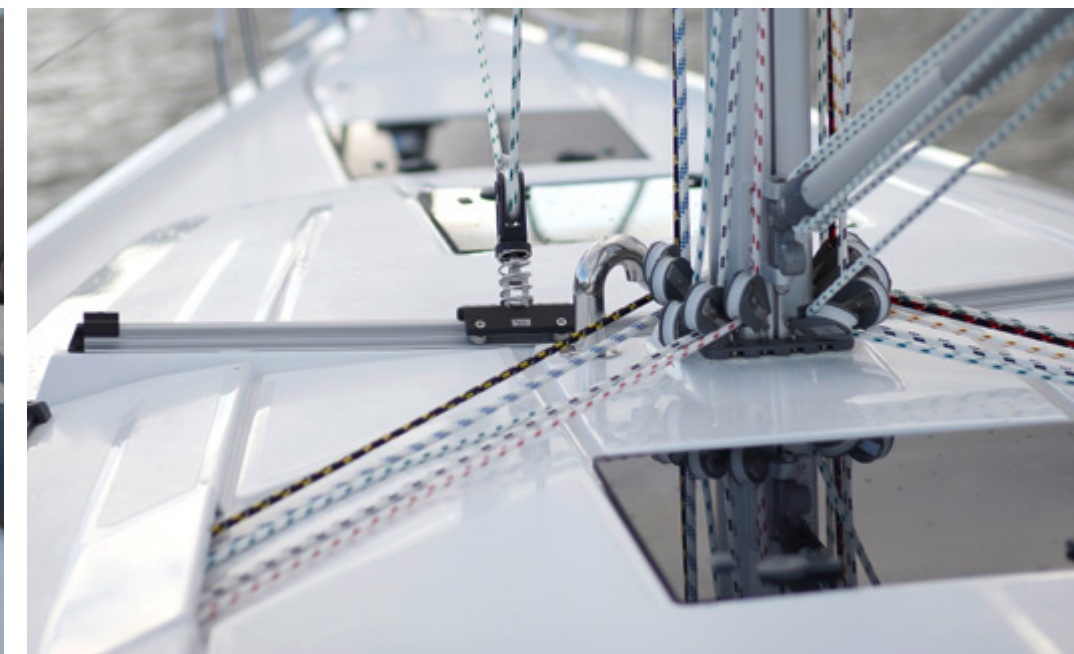
3 Integrated self-tacking jib: tacking with no need for grinding.
