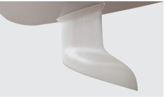
Shallow draft L-keel cast iron, 1,63 m draft
